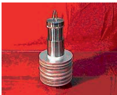
FIG. 31. A typical corrosion test rack with coupons.
