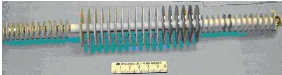
FIG. 35. A coupon assembly used in a research reactor CSP with 32 and 70 mm \phi coupons. The white area between the coupons is a PTFE separator, used to isolate the central stainless steel rod from the coupon and the coupons from one another.
