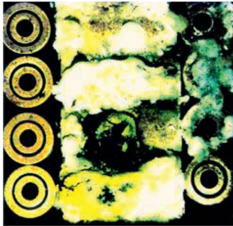
FIG 51. Mark 31A targets in stainless steel bucket storage. Reference [92] provides post-storage metallographic analysis of these aluminium clad, uranium metal materials.
