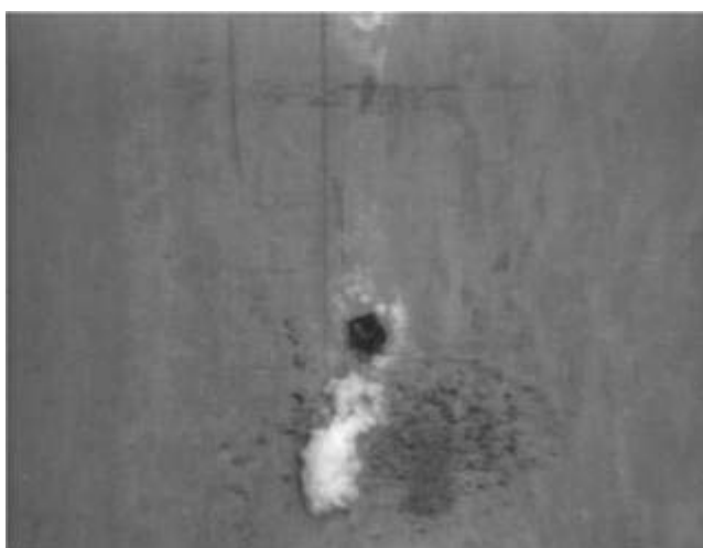
FIG. 6. Through-clad hole from pitting attack on a fuel plate stored for several years in conductive water (nodule removed). Size of hole: about 1 cm.
